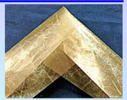
FORMING in any required shape without heating or a temperature between 100 °C to 110 °C and cured after obtaining desired shape.
