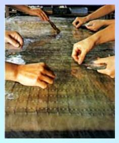
required thermal class binders and hot pressed. Optionally as per application requirement to add extra flexibility, tensile & mechanical strength a variety of reinforcing backing materials are added.
