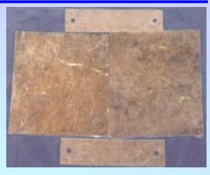
maintain a stable and semi cured state to form dense and flexible sheets so that the sheets can be introduced to forming in any required size without heating.
